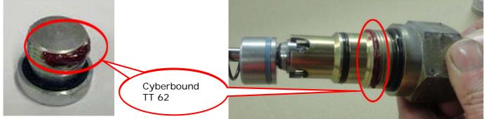
Clean from adhesive residues pressed out from the bore hole after fitting.
